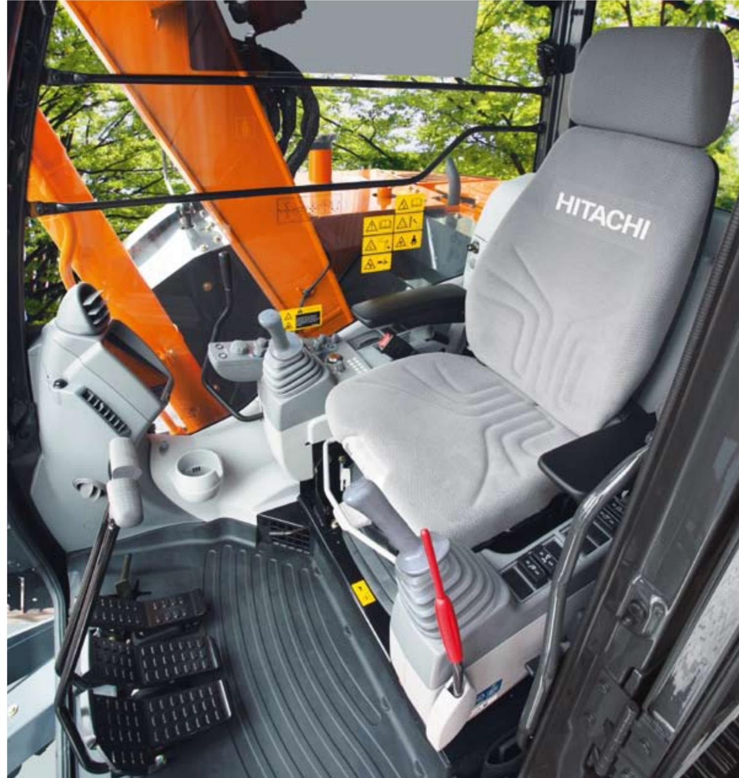
Shown equipped with air suspension seat, attachment pedal, sun visor and blade lever.
