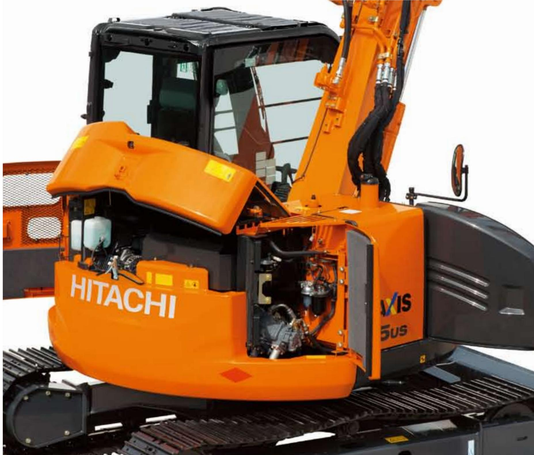
Shown equipped with additional cab rear light, rear view monitor camera and blade.
