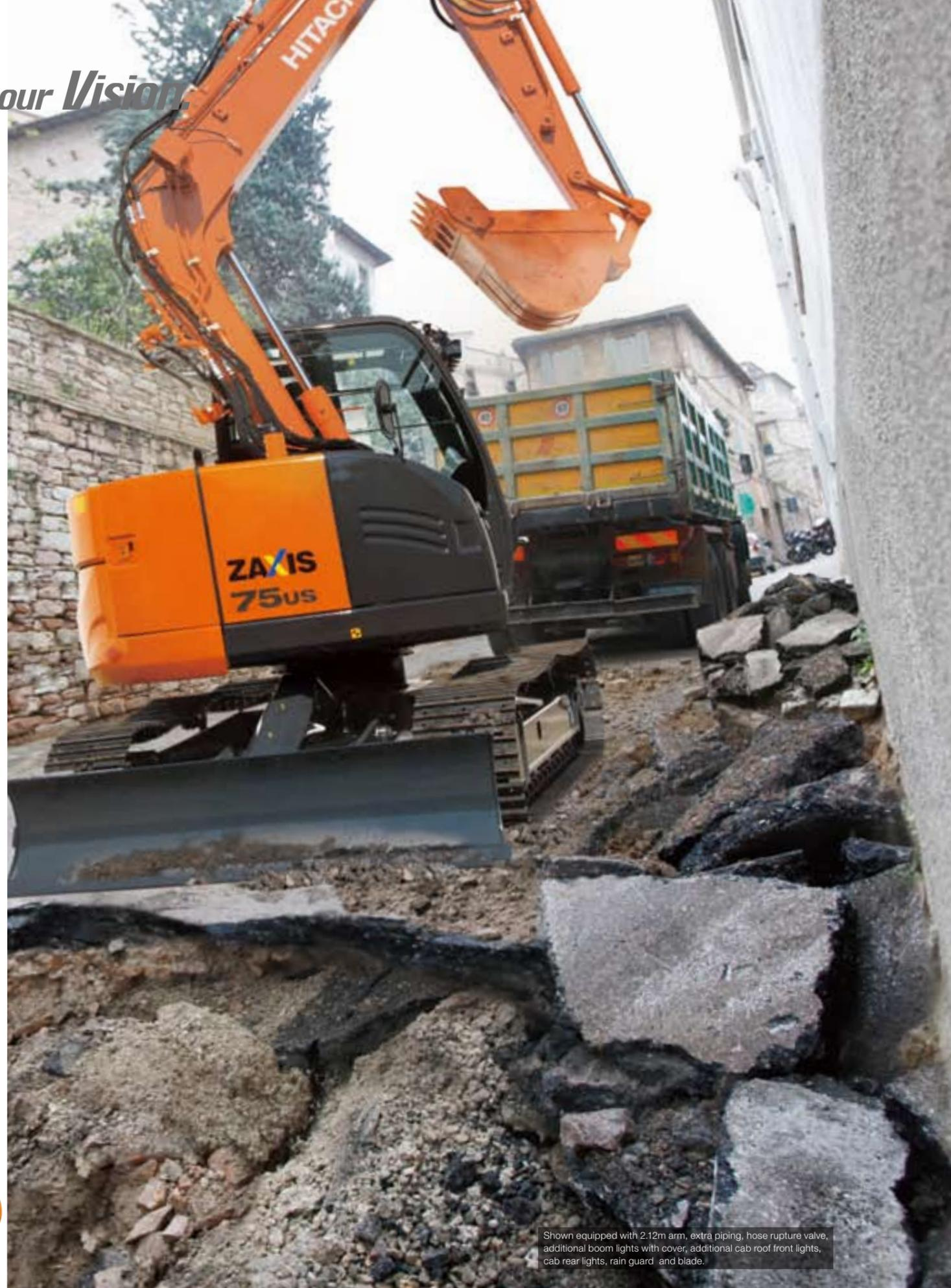
Shown equipped with 2.12m arm, extra piping, hose rupture valve, additional boom lights with cover, additional cab roof front lights, cab rear lights, rain guard and blade.
